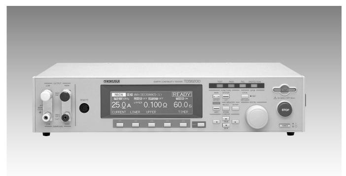
Resistance value: 0.001 to 1.200 $\Omega$  Test Current: 3 to 30 A AC
